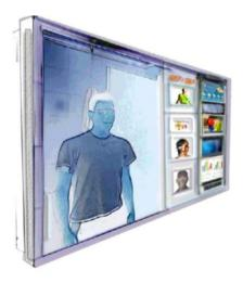
A Smart Health Mirror will utilize Edge Computing, RGB and IR cameras to monitor unobtrusively vital signs, motions and activity
