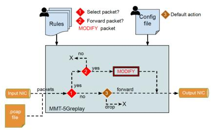
5GReplay's main architecture: Incoming network packets filtered according predefined defined rules that determine which packets are to modified, forwarded or dropped before being sent to the output NIC.
