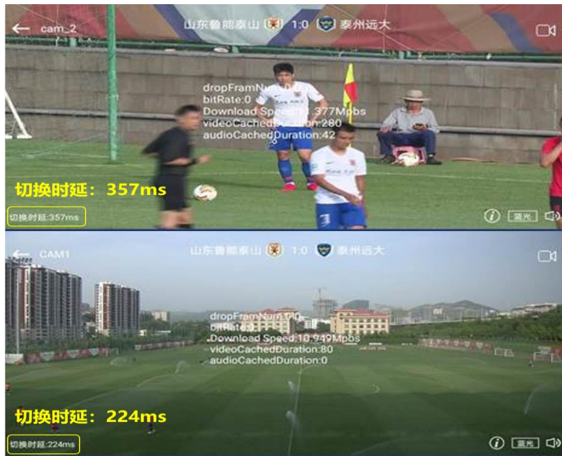
Picture 2 - Test on the switch delay of multiple cameras: ~ 290ms
