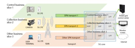
Picture 5 – 5G Smart Grid Slicing Solution
